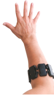
Figure 7.2: Myo Device : Myo install on user's arm, it will detect the electronic signal of muscle.
